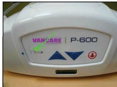
Figure 4C - When the lift has been turned "ON", the indicator light will turn green.
