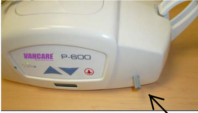
Figure 15A - Gray rubber grommet located on front right side of the lift. Rubber airline is not connected. Note ridge on grommet.
