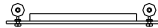
"H" SYSTEM TROLLEY SET USED ONLY WITH "H" FRAME AREA COVERING SYSTEM
