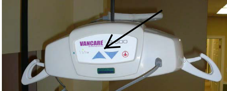
Figure 14A –Lift showing DOWN button located on front right side of lift.
