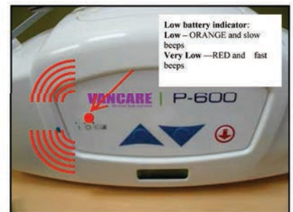
Figure 4D - If the indicator light is ORANGE or RED in color then the batteries of the lift are low and should be charged.
