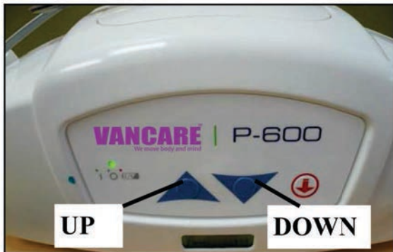
Figure 5C - Front Panel showing raising/lowering buttons
